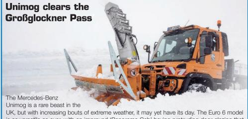
UK, but with increasing bouts of extreme weather, it may yet have its day. The Euro 6 model is as versatile as ever, with an improved 'Panorama Cab' having protruding door glazing that allows a direct rearward view. It also has a 'synergetic traction drive' called Easy Drive, which lets the driver switch from hydrostatic to mechanical drive smoothly while on the move. The 272bhp engine is claimed to use 3% less fuel than its Euro 5 predecessor.
